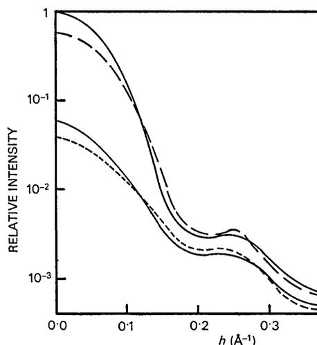
Fig. 1. The upper solid line is the curve which would be seen with pinhole collimation. The lower solid curve is the smear of the pinhole collimation curve. The curve drawn with long dashes is a hypothetical trial function and the curve drawn with shorter dashes is the smear of the hypothetical trial function. These curves are quite representative of the relationships which exist between  $I_0$ ,  $I_{0S}$ ,  $I_{NT}$  and  $I_{NTS}$ .
