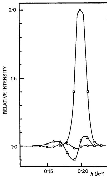
Fig. 2. The curve denoted by the squares is the initial trial function,  $I_{0T}$ , which was used in conjunction with a smeared curve,  $I_{0S}$ , which had a constant value everywhere. After two iterations the third approximation to  $I_0$ ,  $I_{2T}$ , is shown by the triangles. After four iterations the convergence is almost complete as seen by the fifth approximation,  $I_{4T}$ , (circles).
